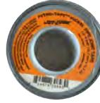
PETRO-TAPE NICKEL is a thick, premium-density tape that permits quick, clean sealing of threaded pipe connections. Its PTFE base provides natural lubrication of the joint, while its nickel filler prevents galling of the threads which is common in stainless steel assemblies. PETRO-TAPE NICKEL contains a gray pigment for easy identification, and distinguishes it from lower density, general purpose thread sealant tapes. HEAVY DUTY - IDEAL FOR MULTIPURPOSE CONNECTIONS, SPECIALLY STAINLESS STEEL.
