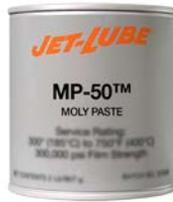
MP-50 was developed for applications where extreme high loads are present, like center bowl lubrication points for rail cars and walking cams for dragline cranes. This product is highly saturated with MoS<sub>2</sub> (Molybdenum Disulphide) in a thick non-melt, grease base for stay put properties. MP-50 is designed to handle high pressure and high heat applications like mandrel forming presses, and is used as a valve stem lubricant for many OEM valve manufacturers.
