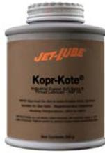
KOPR-KOTE is a combination of copper flake, graphite and other extreme pressure additives, blended into a food grade grease base that helps properly distribute all the components on the surface of the fastener or the metal surface needing lubrication. This particle distribution is necessary to achieve the .15 K-Factor and aids in the break out process by reducing metal-to-metal contact that can cause friction, heat and damage to the threaded surface.
