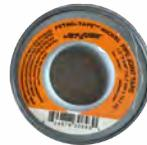
PETRO-TAPE NICKEL is a thick, premium-density tape that permits quick, clean sealing of threaded pipe connections. Its PTFE base provides natural lubrication of the joint, while its nickel filler prevents galling of the threads which is common in stainless steel assemblies. PETRO-TAPE NICKEL contains a gray pigment for easy identification, and distinguishes it from lower density, general purpose thread sealant tapes. HEAVY DUTY - IDEAL FOR MULTIPURPOSE CONNECTIONS, SPECIALLY STAINLESS STEEL.
