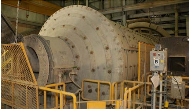
Figure 1. Open gear lubricants are used on equipment such as ball mills (pictured), draglines, kilns, etc.
