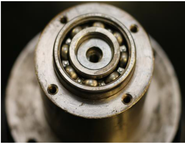
Figure 2. Bearing ready to be packed.
