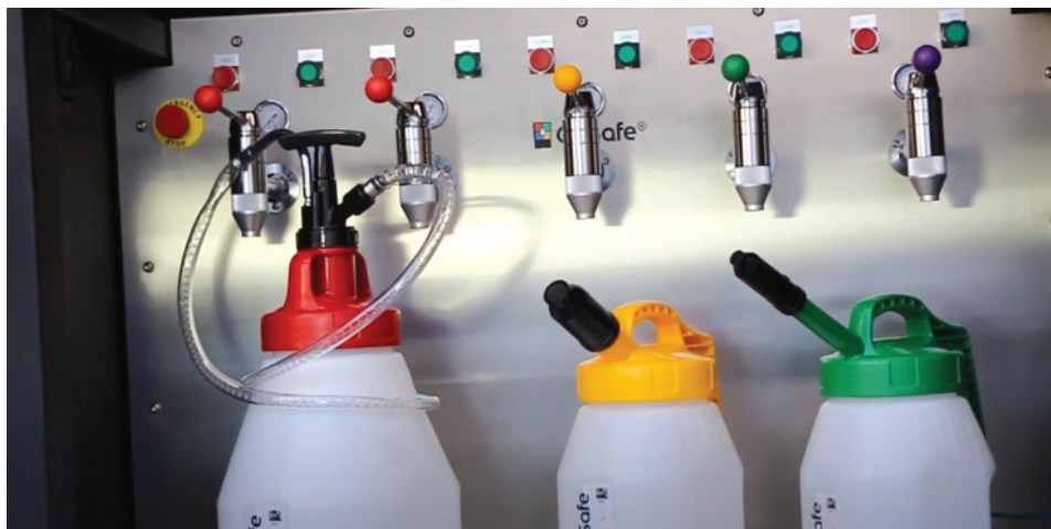
Appropriate lubrication storage equipment and clear labeling of products, through tags, signage or color coding, can reduce the possibility of human error in handling and application.
