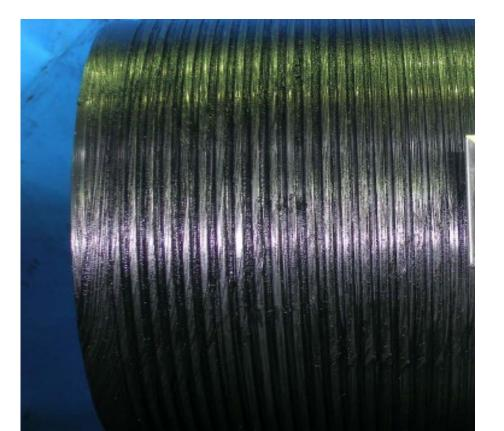
Excess Thread Compound coverage for 8-Round or Buttress Connections
