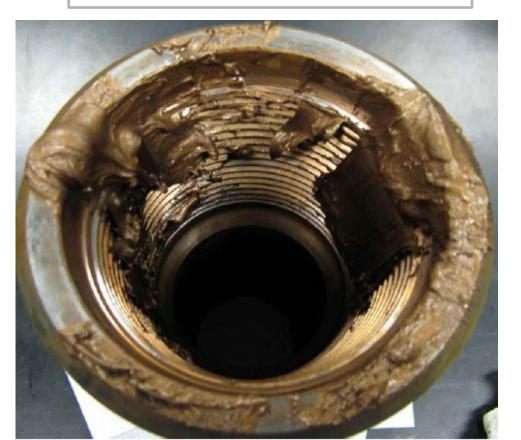
Proper Thread Compound coverage for Rotary Shouldered Connections
